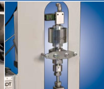
External control of the bleed down valve for piercing process.
