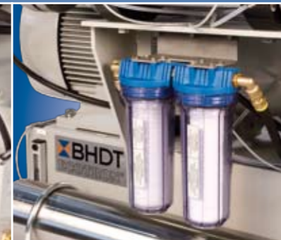
Optimum feed water supply with double filter unit.
