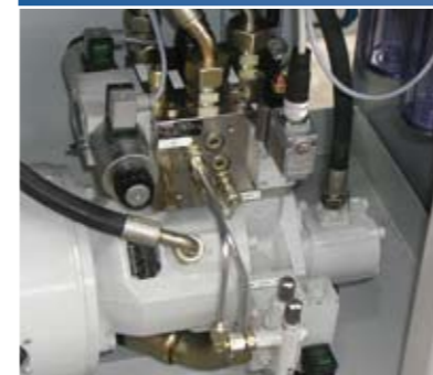
Robust drive hydraulics with axial piston pump and separate gear pump.
